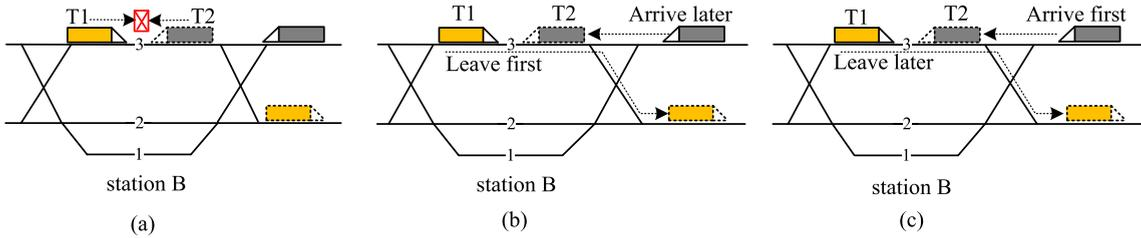
Fig. 5. Conflict resolution when (a) two consecutive trains visiting the same track at stations, where (b) is T1 leave first, T2 arrive later; (c) is T2 arrive first, T1 leave later.
