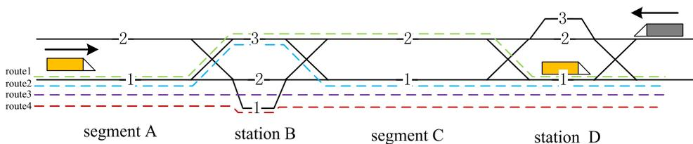
Fig. 4. An example of a railway corridor with four routes.
