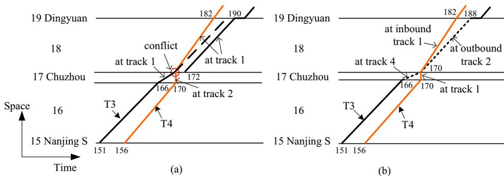
Fig. 15. An illustration of an overtaking: (a) scheduled by In-SSR, (b) scheduled by Co-SSR.
