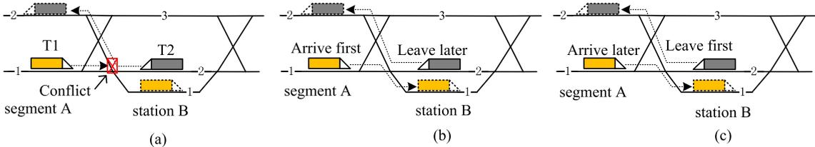
Fig. 6. Conflict resolution when (a) two consecutive trains visiting different track at stations, where (b) is T1 arrive first, T2 leave later; (c) is T2 leave first, T1 arrive later.
