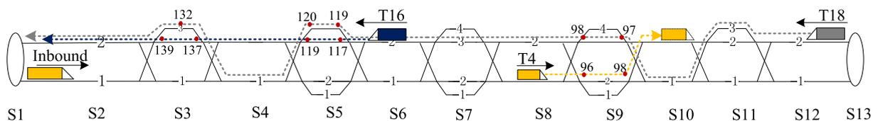
Fig. 11. Illustration of the time and route for two trains in different direction scheduled by Co-SRR.
