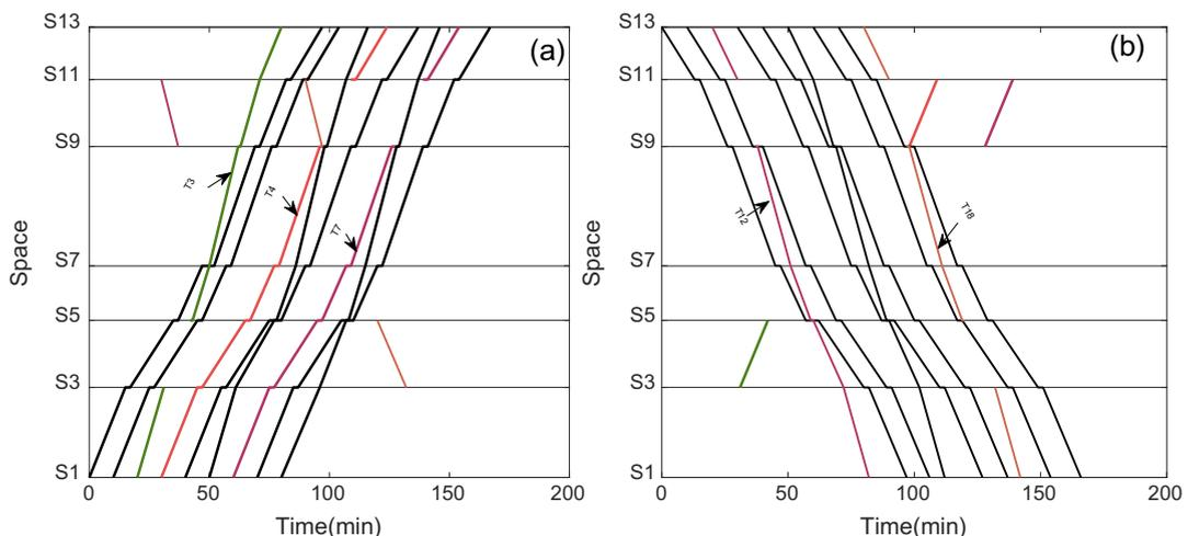
**Fig. 10.** Timetables for the trains in the small-case scheduled by Co-SSR: (a) inbound direction, (b) outbound direction.
