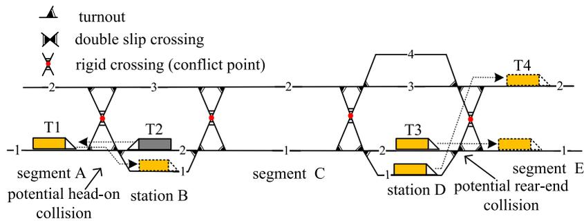
Fig. 7. Examples of crossings in different types of station.
