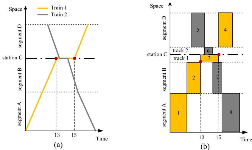
Fig. 2. (a) An illustrative time-space diagram for a railway corridor and its train traffic; (b) the corresponding event diagram, which shows how resources (i.e., segments A-D) are allocated to the trains.
