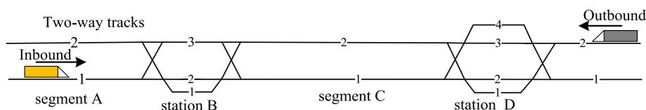
**Fig. 1.** A rail network with two stations and two segments.
