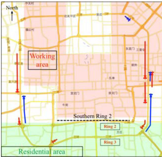
Fig. 14. Congestion map of Beijing. The arrows indicate the major congestions, for which probability of occurrence is over 0.8. The blue arrows: morning rush hours; the red arrows: evening rush hours. The working and residential areas are roughly plotted according to the findings in Dong et al. (2015).
